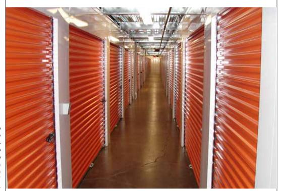
This lower level of a two story conversion has no ceiling and the lights are installed directly to the floor deck. A two story conversion with roll-up doors on both levels requires a 18' interior ceiling height.
