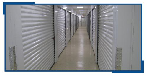
This customer supplied his own ceiling with recessed lights. It is recommended that if this method is chosen, to install the lights every four panels.
