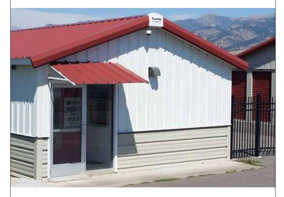
This self-service unit is incorporated into the end of a building using a commercial door and extra window panel. The kiosk enclosure area should be highly visible, well lit, and camera equipped.
