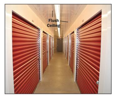
w. A bright white flush ceiling covers all interior duct work and completely encloses the corridor, resulting in a clean, finished look. Lights can be installed directly to the ceiling panel.
