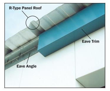
The screws at the eave are located outside the building to prevent roof leaks. The eave trim covers the eave angle and roof screws for a clean, finished look. This feature is standard on all Trachte buildings.
