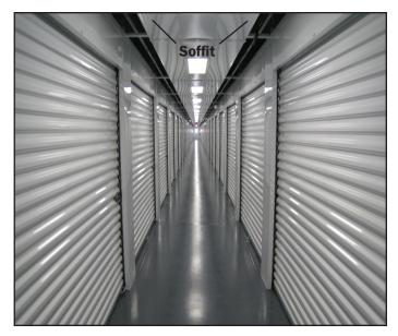
x. A soffit ceiling is recommended if using door alarms. This gives access to the alarms for maintenance purposes. Trachte can supply a LED lighting system, which is recommended.
