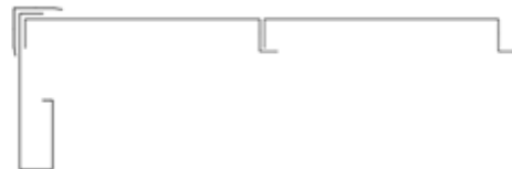
top view, corner assembly with flush panels
